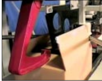
Simple yet efficient flap folding method automatically tucks both top major flaps.
